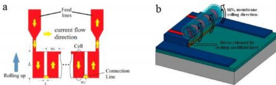
(a) A pattern of conduction strips on a 2D nanomembrane, with arrows indicating the direction of current flow. (b) A nanomembrane rolls up due to stress release. Image credit: Wen Huang, et al. ©2012 American Chemical Society
