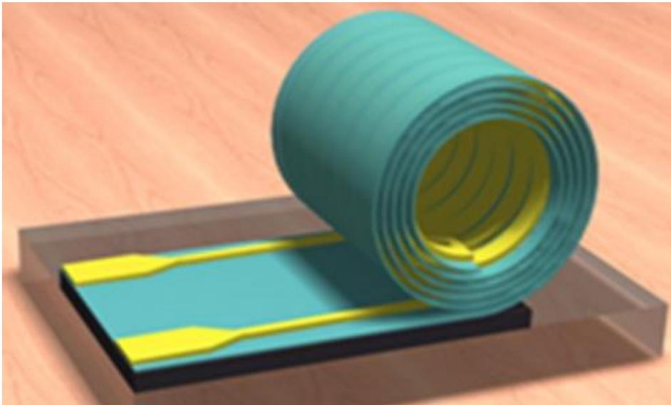
Scientists have designed a 3D inductor that rolls up from a 2D nanomembrane. The inductor offers a better performance and smaller footprint than conventional inductors. Image credit: Wen Huang, et al. ©2012 American Chemical Society
